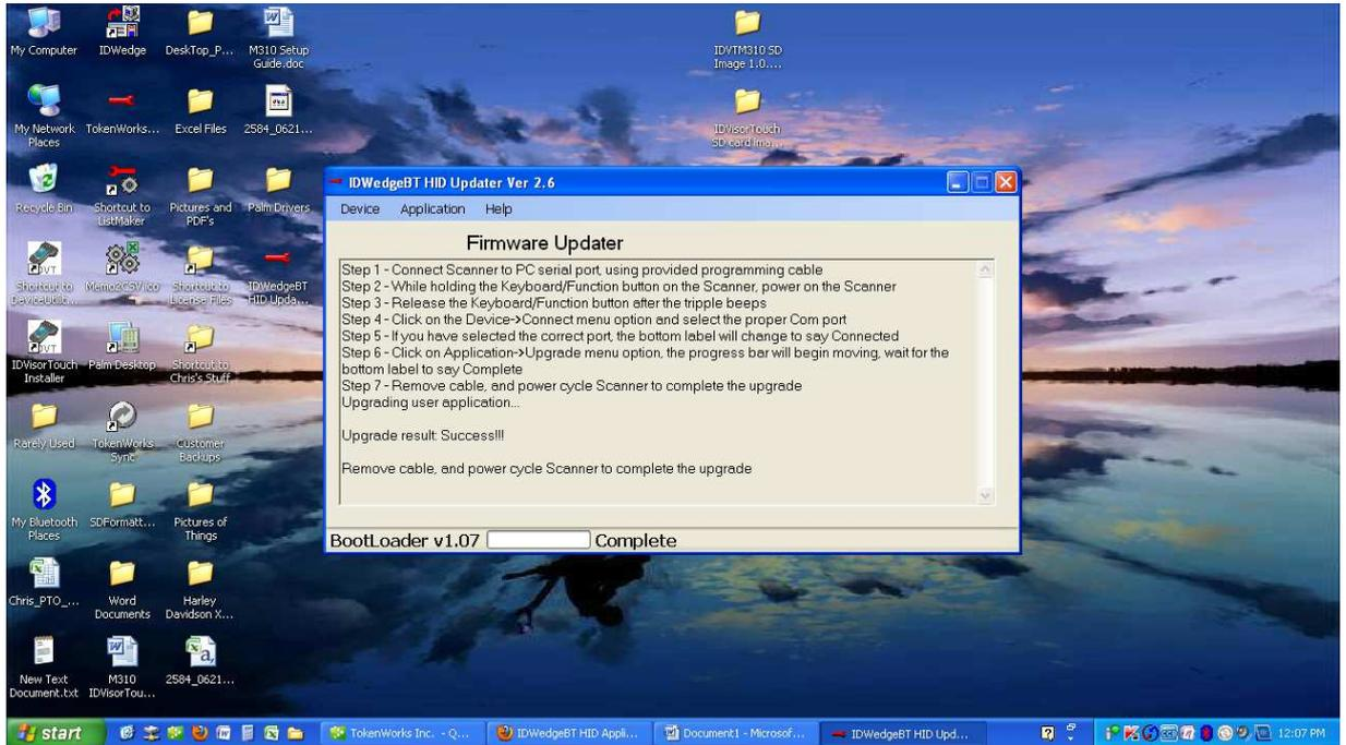
17. The final step is to disconnect the scanner and power cycle it. If it does not automatically turn off after being disconnected, turn it off and then on. It will show a series of blue lights by the battery button. Your scanner should now be ready to go.
