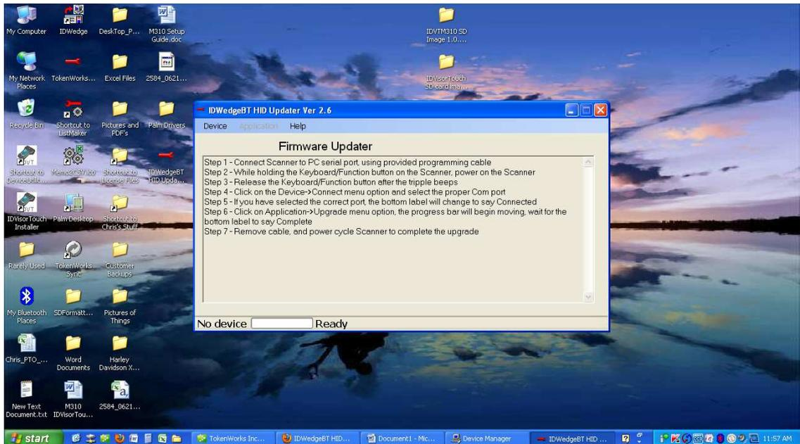
11. Hold the **Keyboard** button as you plug the IDWedge BT ID scanner into the programming cable. It should automatically turn itself on. Now select **Device** from the top menu and select **Connect**:
