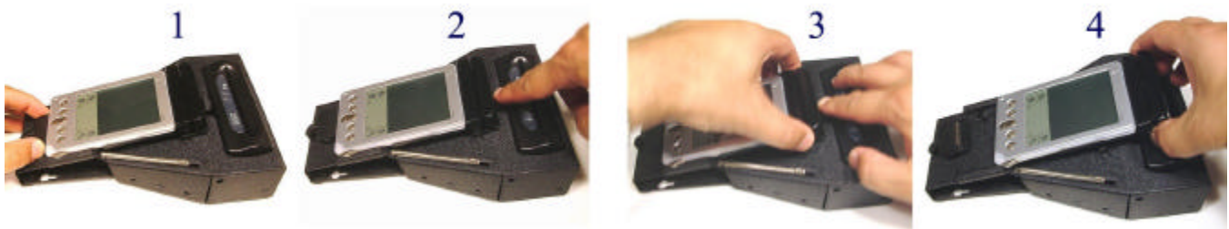
Removing Handheld from Bar Code Reader Cradle Diagram
